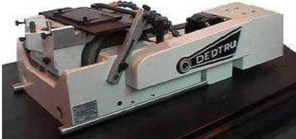
The **Model C6** can be used for through-feed, infeed and secondary operations for larger parts and has a 6 inch regulating roll.
