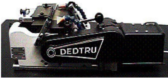
The **Model C** can be used for through-feed, infeed and secondary operations and has a 4 inch regulating roll.
