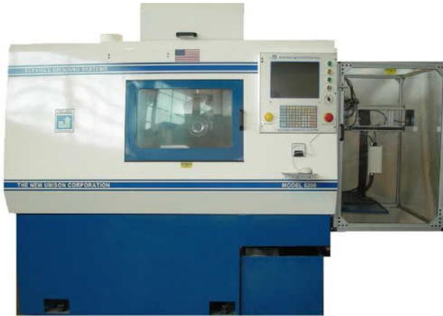
The New Unison **Model 8350** is an Axis CNC production grinder equipped with an automated loader, and a self contained coolant system.
