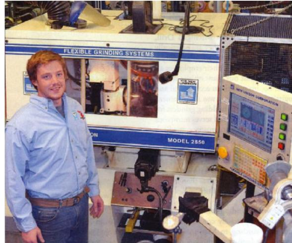
He added that the toolmaker only removes a small cross-section of material when grinding microdrills, and that wear on the grinding wheel is negligible. "It's not the same as huge stock removal--- we probably damage more wheels than we use up".
