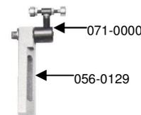
**Horseshoe Double Pressure Roll Assembly** supplied with two 1/2" diameter rolls. This assembly is applied when it is desirable to capture the part at both ends and grind in the center. The rolls can be individually canted to push (for compression) or to pull so that very fine parts can be ground under tension.
