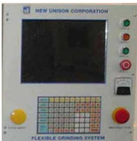
The UPC utilizes the Windows 7™ Operating System and the software monitors all critical machine functions and alerts the operator to problems encountered during grinding. Errors are tracked and logged within the machine's control to easily identify a problem. The Model 1500 can be networked and monitored via the internet or through a central data collection point.
