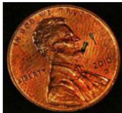
Two examples of the tiny parts ground at M&S are a 0.058" long barbellshaped locking pin for a heart valve repair device and an H13 tool-steel core pin for a medical product mold which is 0.090" long with diameters of 0.003" and 0.012".
