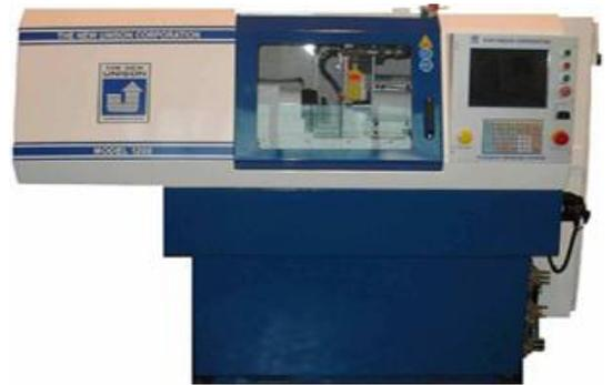
The Model 1500 is a rigid production grinding system designed to grind round & non-round OD shapes, as well as contours and peel grinding. Featuring Unison's proprietary grinding technology, the Model 1500 is capable of meeting the most demanding grinding applications with fast cycle times.
